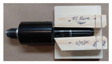
Cut the square stock in half. Place the Morse taper on your live center on the plywood, and glue the two pieces of square stock to the plywood, making sure they are snug against your live center. I shot a couple of nails in to hold them in place while the glue dried.
