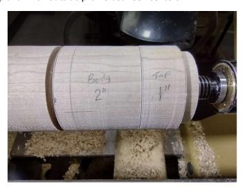
Remove tailstock live center and finish end of top ("Charmin jam chuck" may be required depending on fit).
